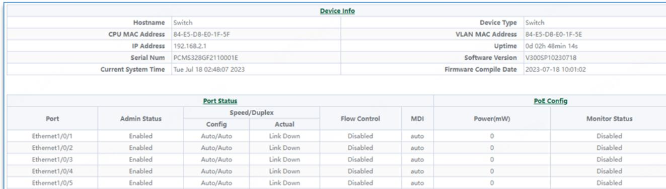
This screenshot shows the "Device Info" and "Port Status" sections of the System Homepage. The "Device Info" table includes fields for Hostname (Switch), CPU MAC Address (84-E5-D8-E0-1F-5F), IP Address (192.168.2.1), Serial Num (PCMS328GF2110001E), and Current System Time (Tue Jul 18 02:48:07 2023). The "Port Status" table lists ports 1 through 17, all of which are currently Link Down. The "PoE Config" table indicates that ports 1 through 17 are not supported.
