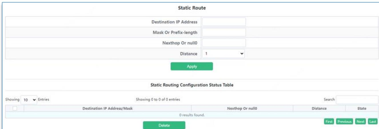
The screenshot shows a 'Static Route' configuration form with fields for Destination IP Address, Mask Or Prefix-length, Nexthop Or null0, and Distance (set to 1). Below is a 'Static Routing Configuration Status Table' with columns: Destination IP Address/Mask, Nexthop Or null0, Distance, and State. It shows 'Showing 0 to 0 of 0 entries' and '0 results found.' Buttons for 'Apply' (green), 'Delete' (red), and navigation ('First', 'Previous', 'Next', 'Last') are at the bottom.
