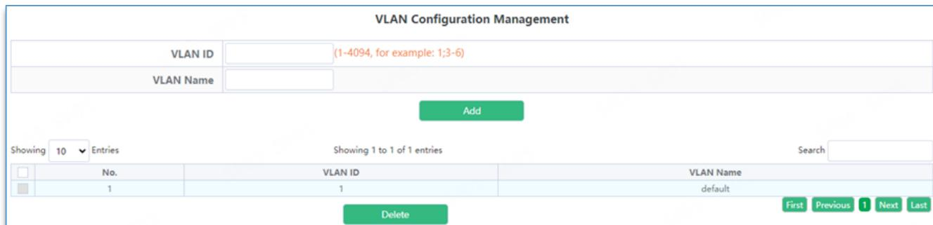
The screenshot shows the 'VLAN Configuration Management' interface. At the top, there are input fields for 'VLAN ID' (containing '1-4094, for example: 1;3-6') and 'VLAN Name' (empty). Below these are 'Add' and 'Delete' buttons. On the left, a dropdown menu shows 'Showing 10 Entries'. The main area displays a table with one entry:
